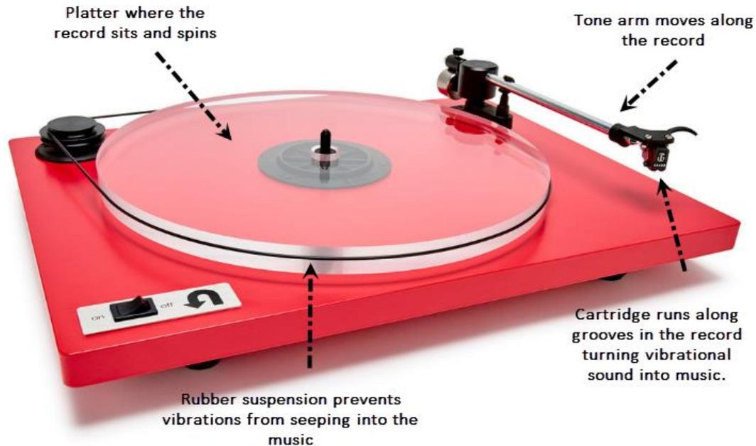
The device comes ready to play out of the box. Users only need to turn it on and lower the tone arm to play a record. Each turntable comes with a pre-installed, adjusted cartridge, which works to convert vibrational energy from the record into analog sound. Additional accessories also include RCA cables, a dust cover to protect the records, and a felt mat.
